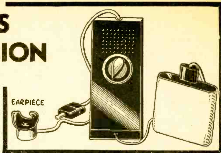
Component parts of a portable hearing aid.
